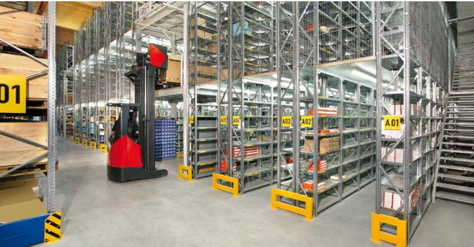
*The warehouse has a ground surface area of 900 square metres and is divided up almost quadratically. This manual order picking warehouse has a 3-tier META HIGH-CLIP® shelving system.*
