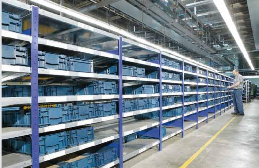
**META QUICK® inclined shelving is optimal for boxed goods and crates; the goods slide automatically down to the take-out side**
