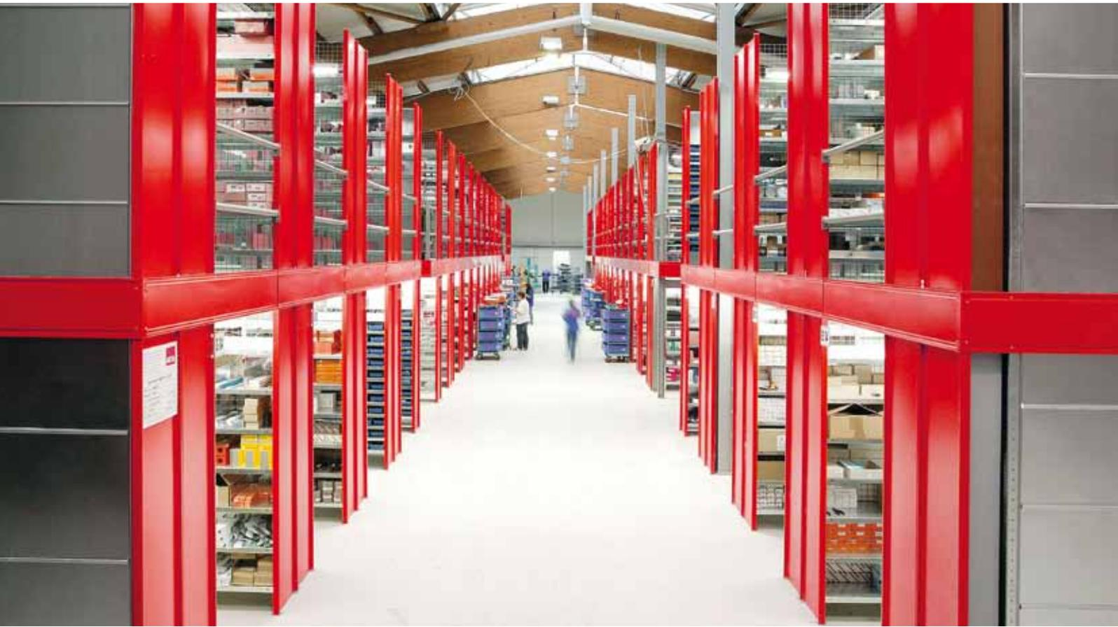
*This META QUICK® shelving system is extended upward with 2 tiers on one side and 3 tiers on the other*
