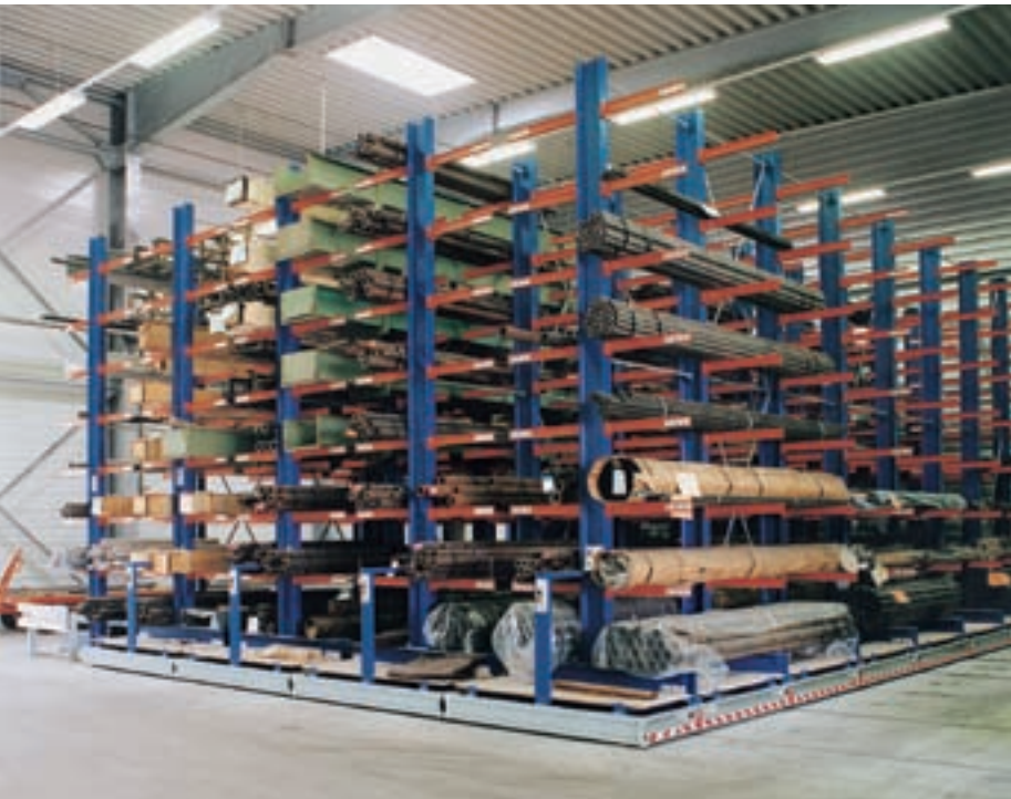
Cantilever, blocs mobiles
